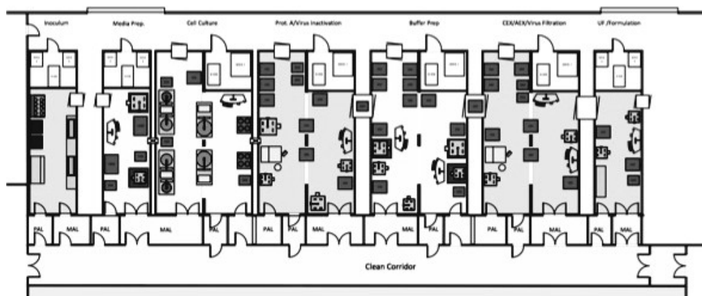
Figure 8: Bioprocess layout with segregated unit operations
